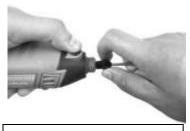
5. Push the fastener, rotate to tighten the grip chuck.
